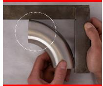
**Other** short radius bends are typically produced using the pressing method which means the bends are not able to be made with any straight sections.
