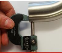
**Other** bends are typically bent using heavier wall tube and then polished back, resulting in variable wall thickness. This internal polishing can also hide defects on the inside of the bends.
